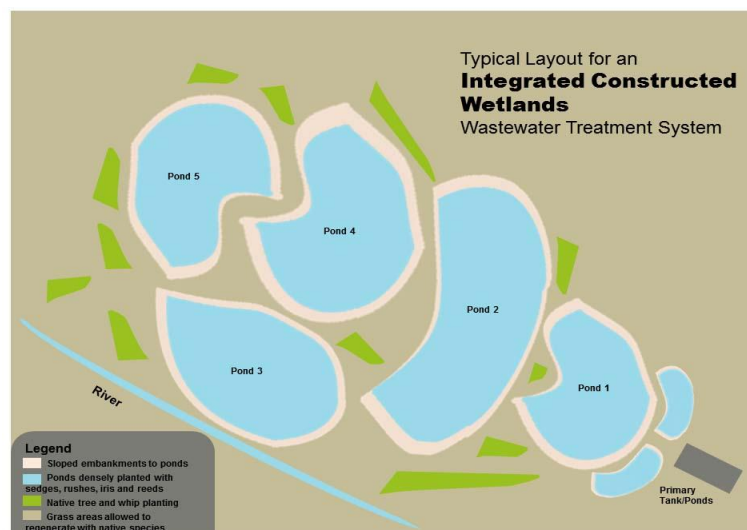
Figure 5.13 - Integrated constructed wetlands
