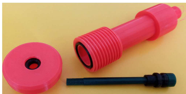
Fig. 7. Second iteration of a 3D printed linear actuator and finished parts of the second iteration of a 3D printed linear actuator
