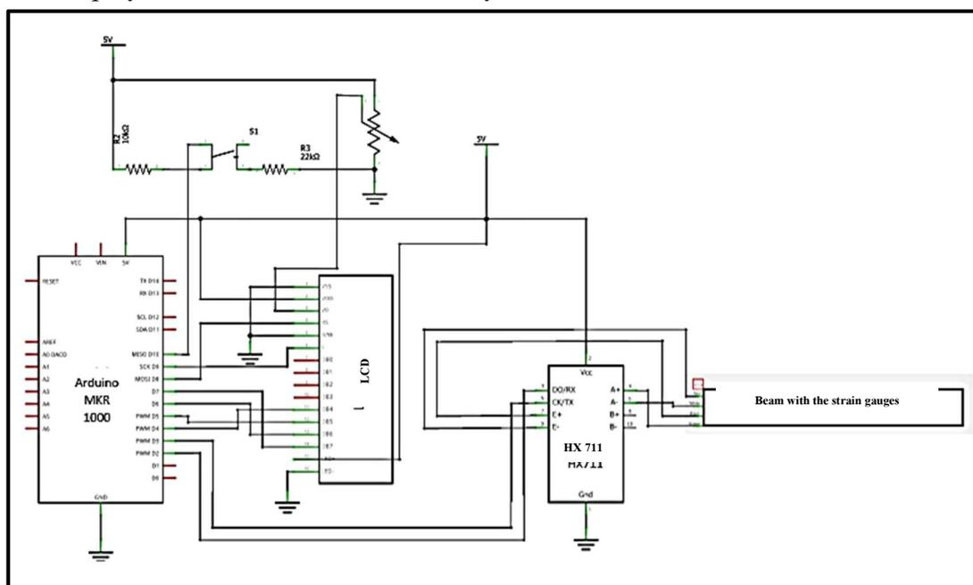
Fig. 10. Final measuring chain [16]
