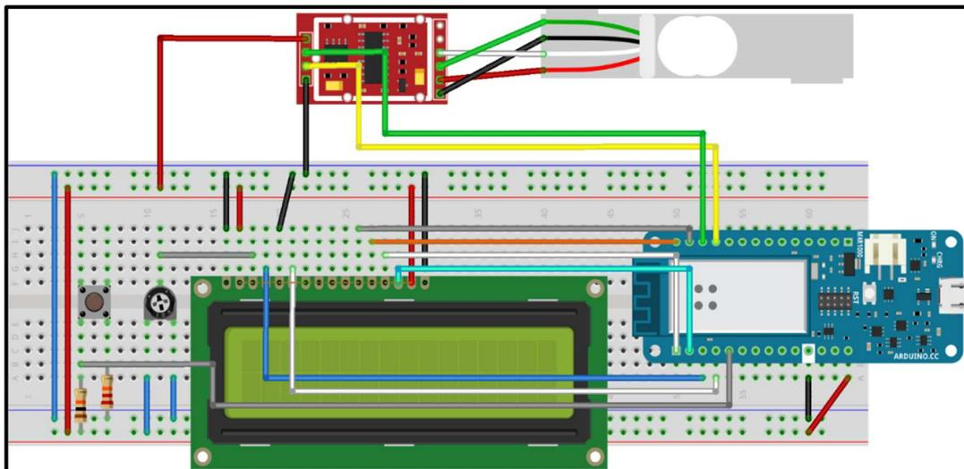
Fig. 11. Equipment connection design from Fritzing [16]
