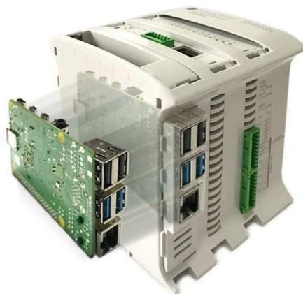
*Fig. 6. PLC based on RPi [7]*
