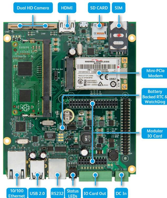
Fig. 4. Industrial IoT Integrator Board (MyPi) [6]
