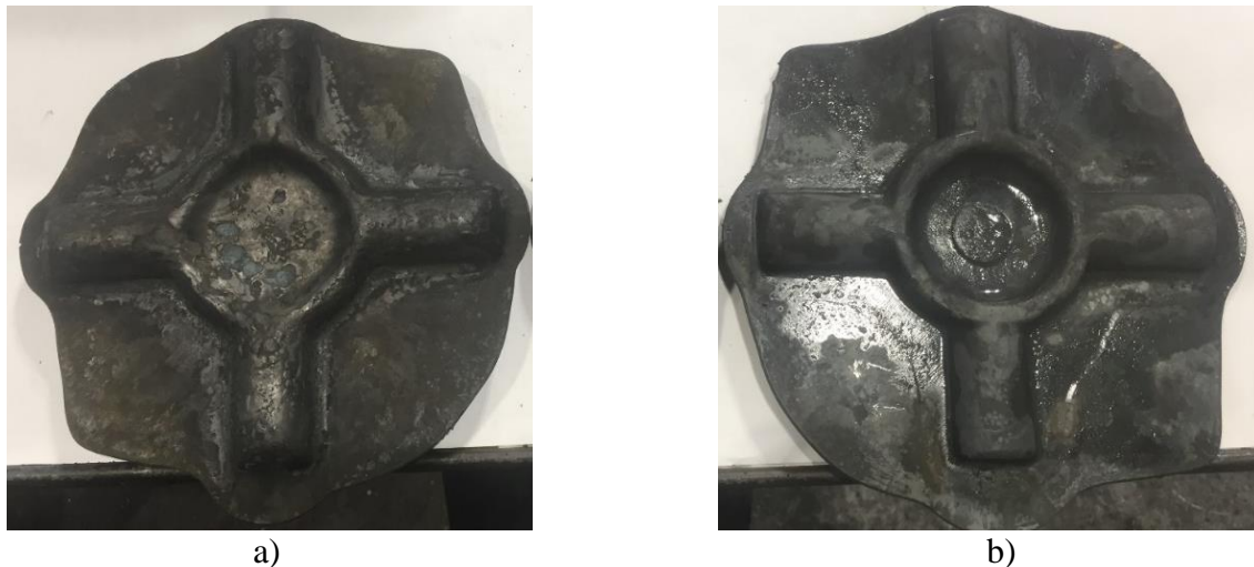
Fig. 3 – Photo of the actual preform (a) and finished (b) forged parts using proposed preform shape (no material flow defects observed).
