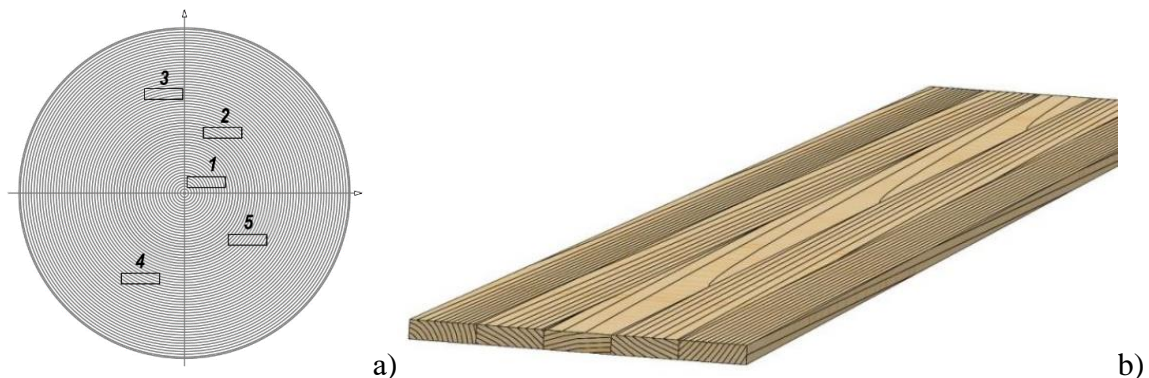
Fig. 2 – the position of the lumber in the log (a); the projected view of the board glued together sequentially from lumber No. 1-5 (b).
